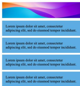
Figure 7 Example of fluid grids with CSS multi-column layout and one media query
